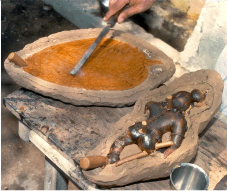
A new bronze still embedded in its clay encasement. http://www.tms.org/pubs/journals/JOM/0210/Pillai-0210.html
